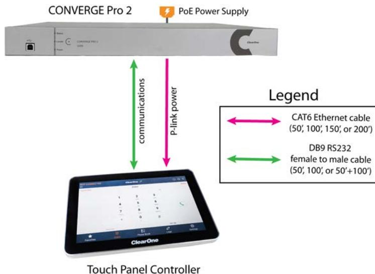
**Connection Note:** Maximum CAT 5e/6 cable length for P-link connections is 200 ft (61m). Maximum RS232 cable length is 150 feet (46m).
