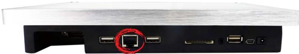
If you're using DHCP, no further configuration is required. To use a static IP address, you must configure the Touch Panel Controller Ethernet settings. See [Configuring Ethernet Settings \(VoIP/Telco\)](#) for more information.
