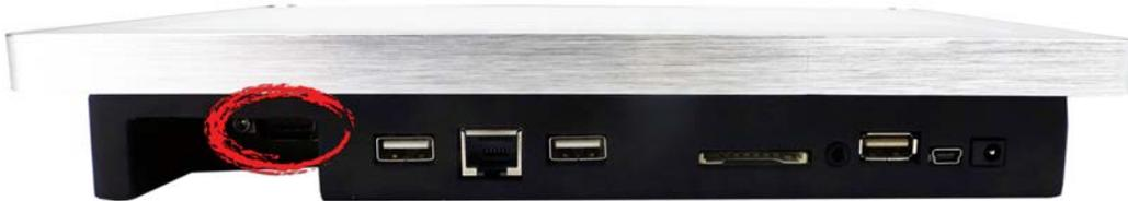
You can connect directly using a standard RS232 serial cable for communications:
