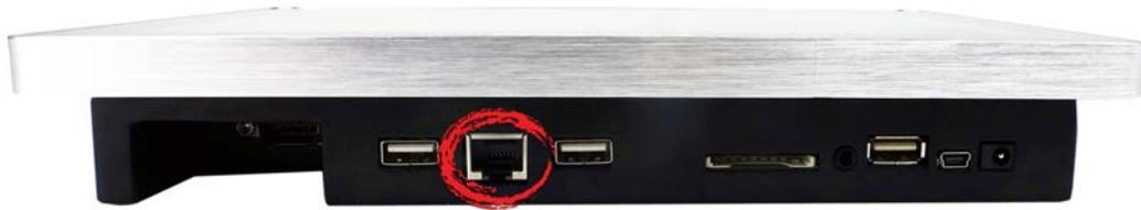
By default, the Touch Panel Controller connects to the network using DHCP. If you're using DHCP, no further configuration is required. To set a static IP address, follow the steps below.
